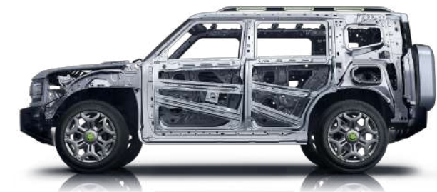
Steel cage body structure
