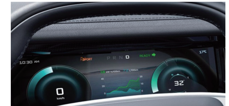
The 10.25-inch digital instrument panel
